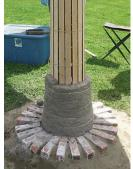
I've been building my furnaces from a traditional mix of clay and sand that has many benefits over modern furnace materials, and this approach has resulted in iron and steel that is easier to refine. Processing and using this material has given me many insights into the how and why of Viking weapons.
